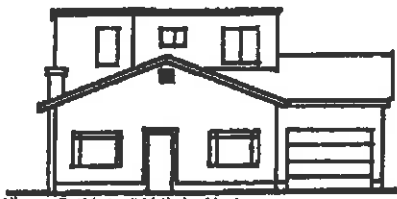
Avoid - Roof does not follow existing roof slopes
